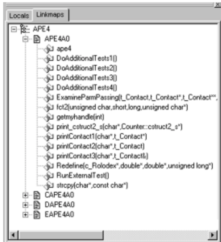
Figure 1: The Linkmap Window uses a tree structure to display the files and functions that belong to a program.
